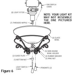
**CAUTION:** Never use pliers to tighten bottom nut against the bowl. A broken or damage bowl will most surely result.
